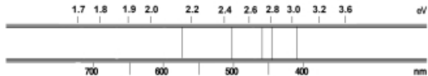
Figure 5-2: The light emission spectrum of hydrogen and nitrogen.
