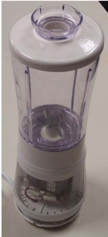
Figure 1: Blender with cut-out view for students to see inside when motor is running
