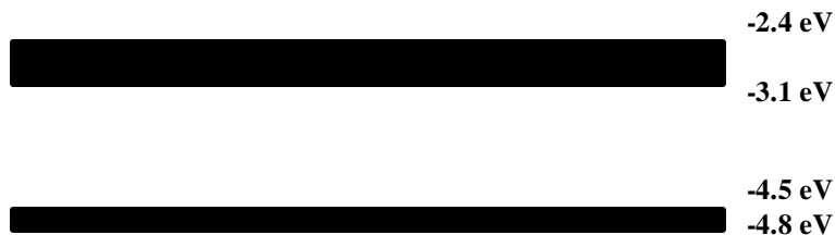
Figure 4-3: Energy Bands and Gap of the LED Solid
