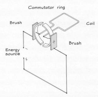
Many motors use splitring commutators. Each end of the coil is attached to half of the ring. An electric insulator separates the two halves. Two metal contacts, called brushes, are attached to an energy source. As the commutator rotates. each half alternates contact with the positive and negative brushes. This leads to a current in the coil that reverses direction every half revolution.
