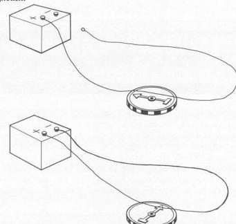
Oersted placed a long wire parallel to a magnetic compass. When an electric current moved through the wire, the compass rotated so that it was perpendicular to the wire.
