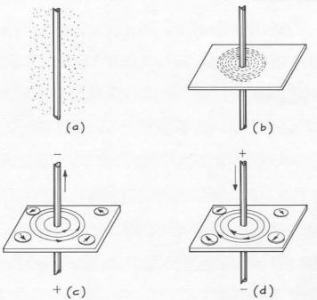
Iron filings and magnetic compasses trace out the magnetic field produced by the current-carrying wires. (a) No magnetic field exists in a plane parallel to the current-carrying wire. (b) Perpendicular to the wire, the iron filings arrange themselves in a circular pattern. (c) The magnetic field lines are counterclockwise when the current moves upward and (d) clockwise when the current moves downward.
