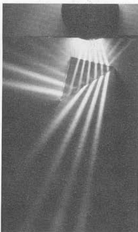
Figure 15-21 Light is refracted as it strikes the glass surface of a prism.
